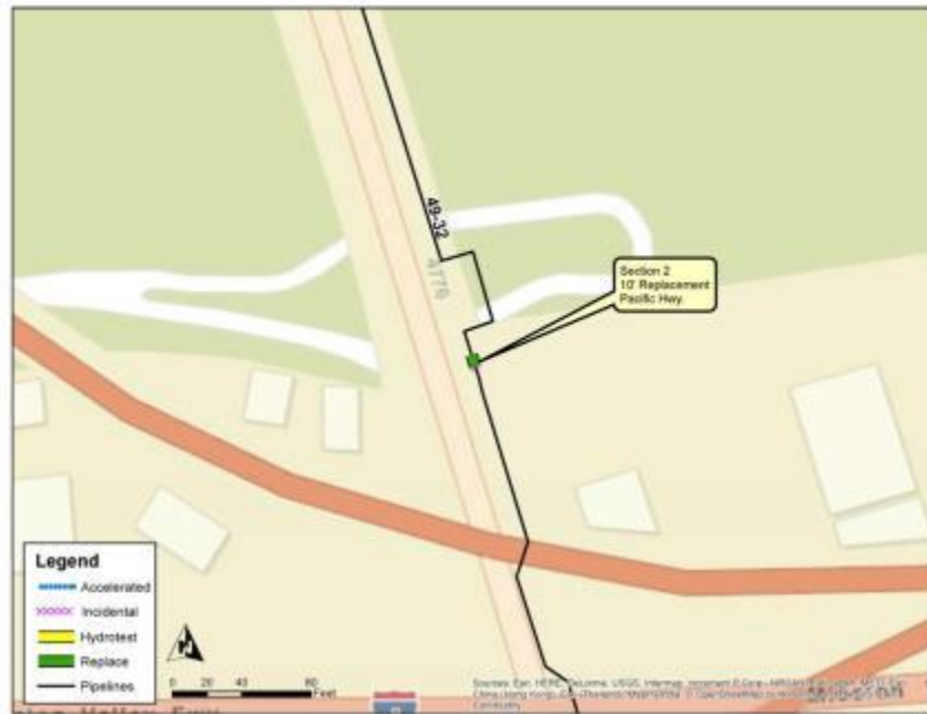
Figure 5: Overview Map of L-49-32 Section 2 Replacement Project
