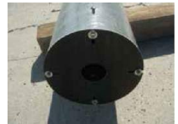
J-BOLTS ON INSIDE OF MODULE
