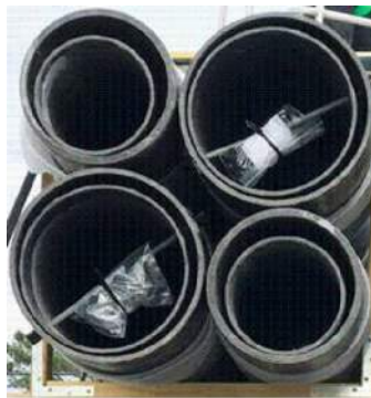
FIGURE 7 NESTING FOR TRANSPORTATION (B)
