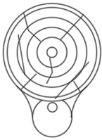
METHOD 1 IMPREGNATED FIBER CONDUIT OF 1/4" MINIMUM THICKNESS
