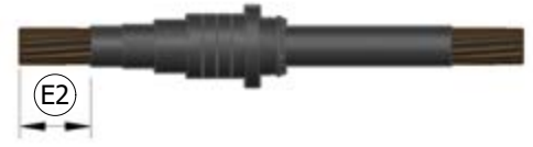
FIGURE 3 WIRE STRIPPING (E)
