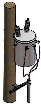
FIGURE 1 TERMINAL CONSTRUCTION (a) ISOMETRIC VIEW
