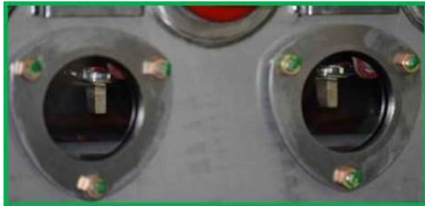
FIGURE 47 VISIBLE OPEN SHAFT (K2) "OPEN"
