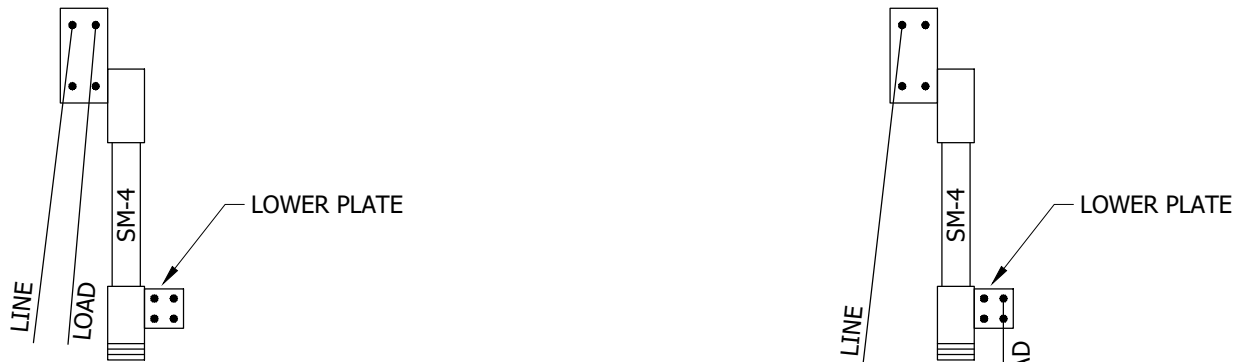
FIGURE 1 XFMRs CONNECTED WITH LOOP FEED SM-4 FUSE IS FOR TRANSFORMER FUSING ONLY AND (B) NOT FOR "LOOP" LOAD
