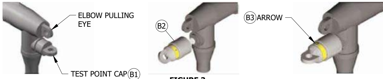
FIGURE 3 PHASE SENSOR BOOT
