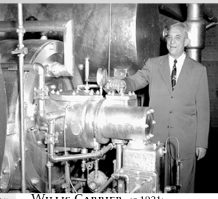
WILLIS CARRIER (c.1921) • "CENTRIFUGAL REFRIGERATION MACHINE"
