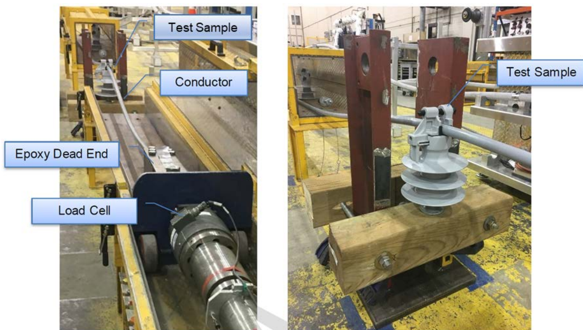
Figure 61. Representative photos of insulator slip test.
