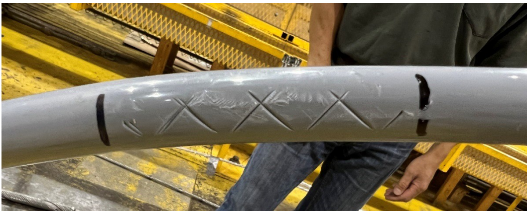
Figure 6-8: Sample 3.1.1 - 17 kV, 1/0 AWG ACSR Condition after Test
