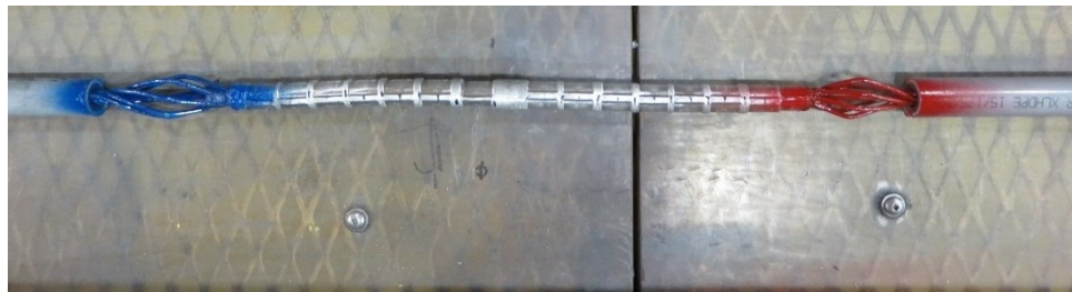
Figure 3-3: ██████ installed on 35 kV 1/0 AWG, 6/1 ACSR
