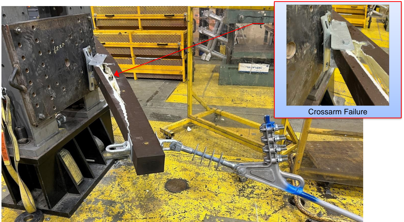
Figure 6-24: Sample 6.3 – Failure Location
